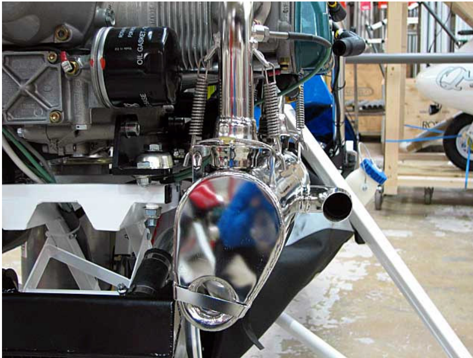
Fig 4 Exhaust springs and backup cable
